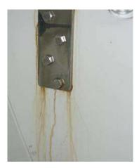
area, but there is still a chance there may be core damage. If any of the core is damaged, remove the damaged area by reefing out the core and replace the area with a WEST epoxy repair kit using the filler to create a paste and then file the hole into shape. Another technique that can help prevent "wicking" of moisture along the stainless plate is apply a strip of metal primer to ensure a bond with the sealant. If any of the chainplate bolts are corroded, they should be replaced.
